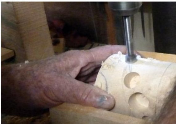
1. Holes were drilled with a Forstner bit.
